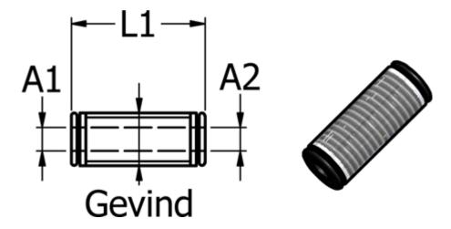
Ext. hose diameter A1 = 5 Ext. hose diameter A2 = 5 L1 = 33.5 Thread = M14x1
